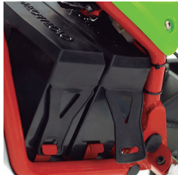
Easy to lock: Elastomer battery cover
